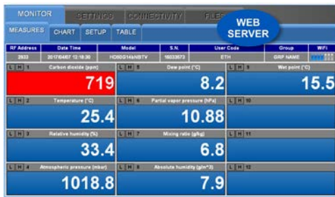
Web server: monitor of measurements with CO 2 measurement in alarm
