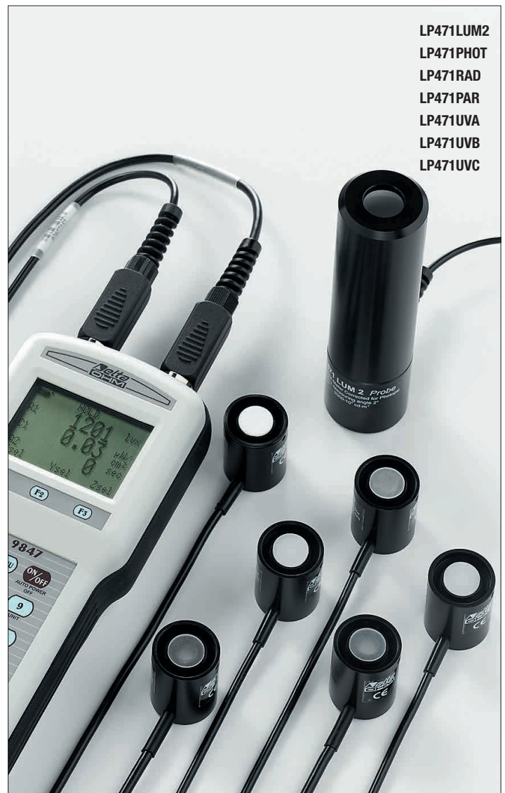
LP471PAR Quantum radiometric probe for the measurement of the photon flow across the chlorophyll range PAR , equipped with SICRAM module.
